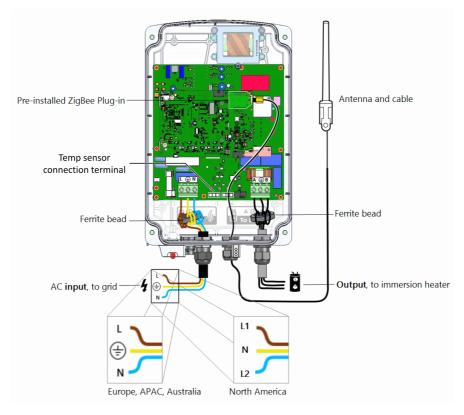
Figure 9: Smart Energy Hot Water wire connections
