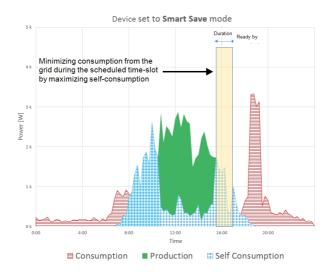
Figure 2: Examples of device operation
