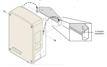
Figure 7: Hanging the device on the bracket
