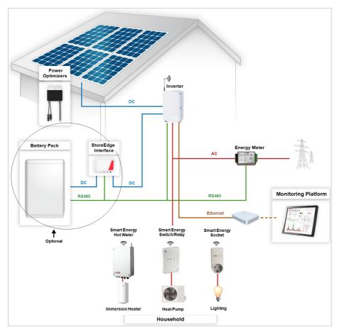
Figure 1: SolarEdge system with Smart Energy products
