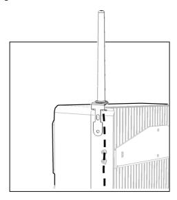
Figure 10: Mounting the Antenna
